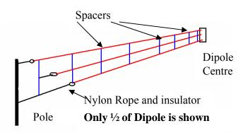
The principle of operation of this multiband antenna is that the rig will automatically select the appropriate resonant dipole at its operating frequency and deliver most of the RF power to it. The theory is that that the other dipoles will have only minimal effect.
